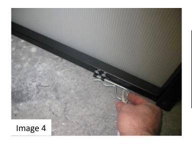
Never move a stack without a safety rope. If the Stack Opens Flat the Top Panels will Fold Back Down and Ruin your Day
