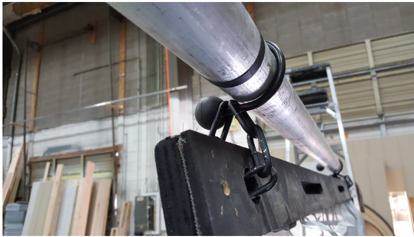
Finished U-bolt hanger
